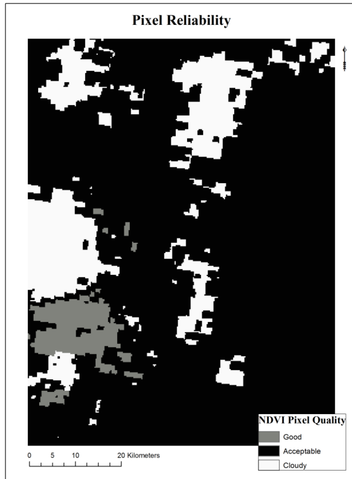
Figure 5.1. 250m NDVI pixel quality assessment layer from MOD13Q1 product of the MODIS sensor
